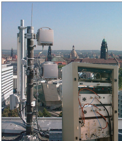
■ Figure 2. Test base station with antennas and microwave link at central site.
