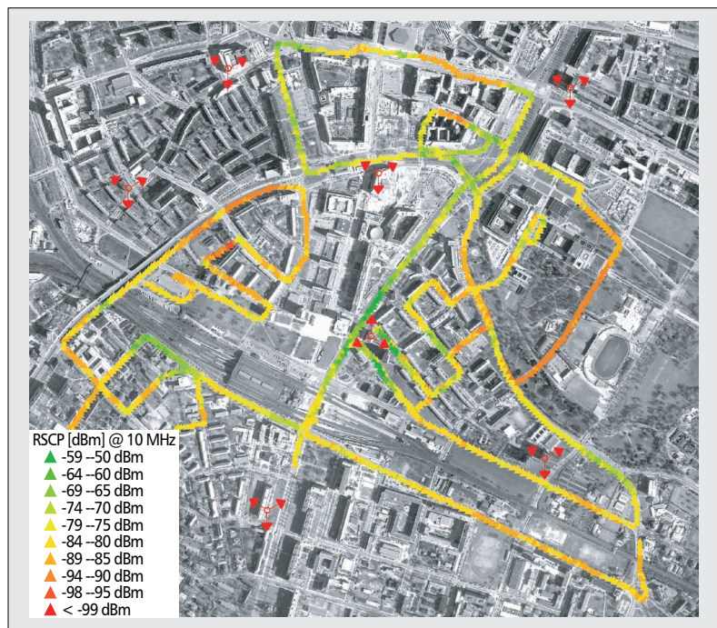
■ Figure 3. Signal coverage of the trial area based on drive tests.
