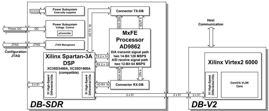
Fig. 2: Block diagram of the DB-SDR Extension module
